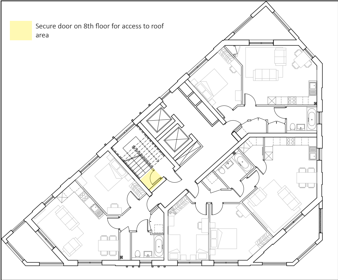
53.1 Additional door in stairwell on 8th floor
