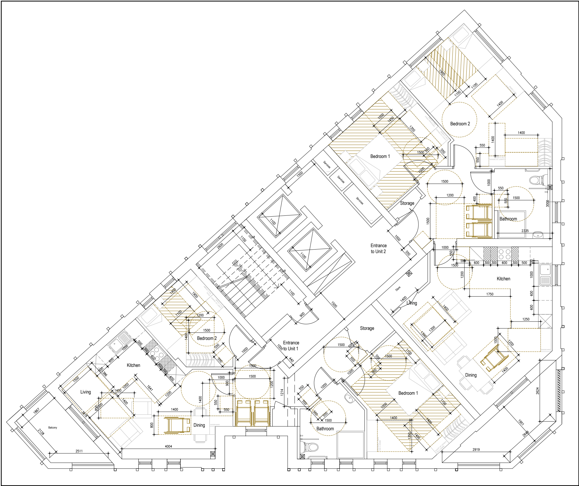
49.1 Part M4(3) compliance for first-floor units
