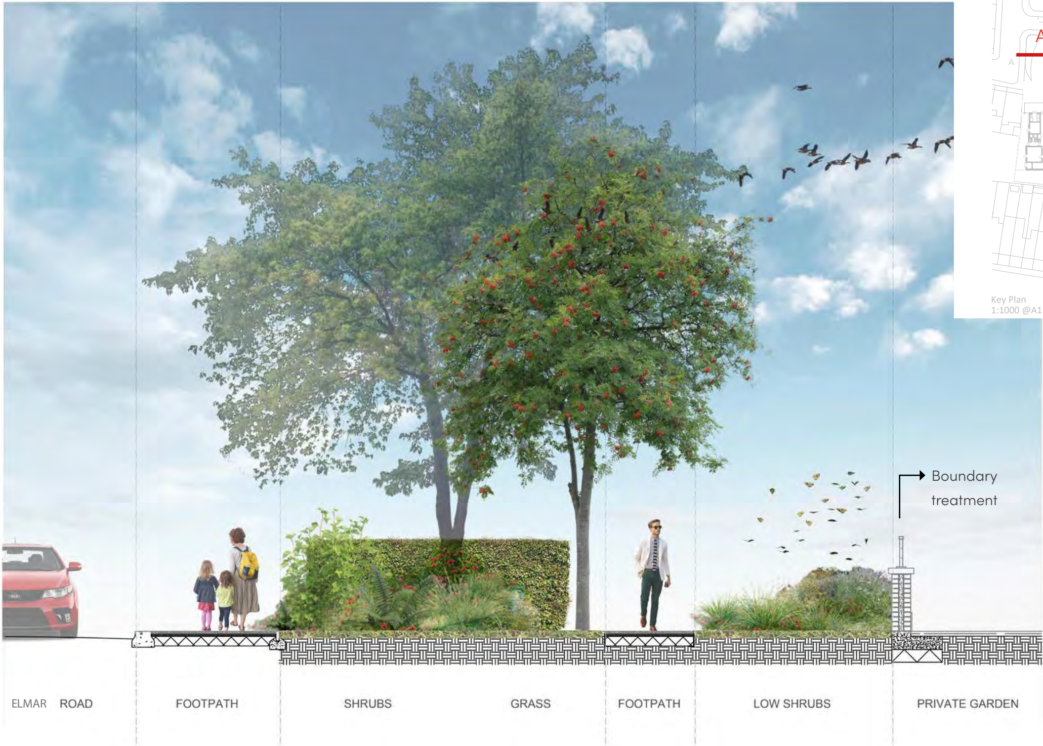
A-A' Section through Green Buffer from road level and boundary treatment to private garden
