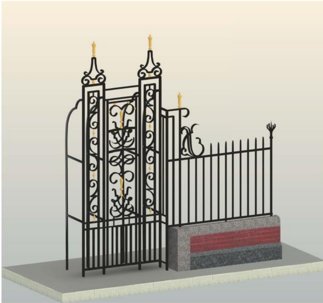
004 – General view of proposed right hand gate support and masonry wall
