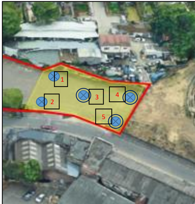
Figure 2: Aerial Image for the Phase 1 Site and the Proposed Borehole Locations and Installations
