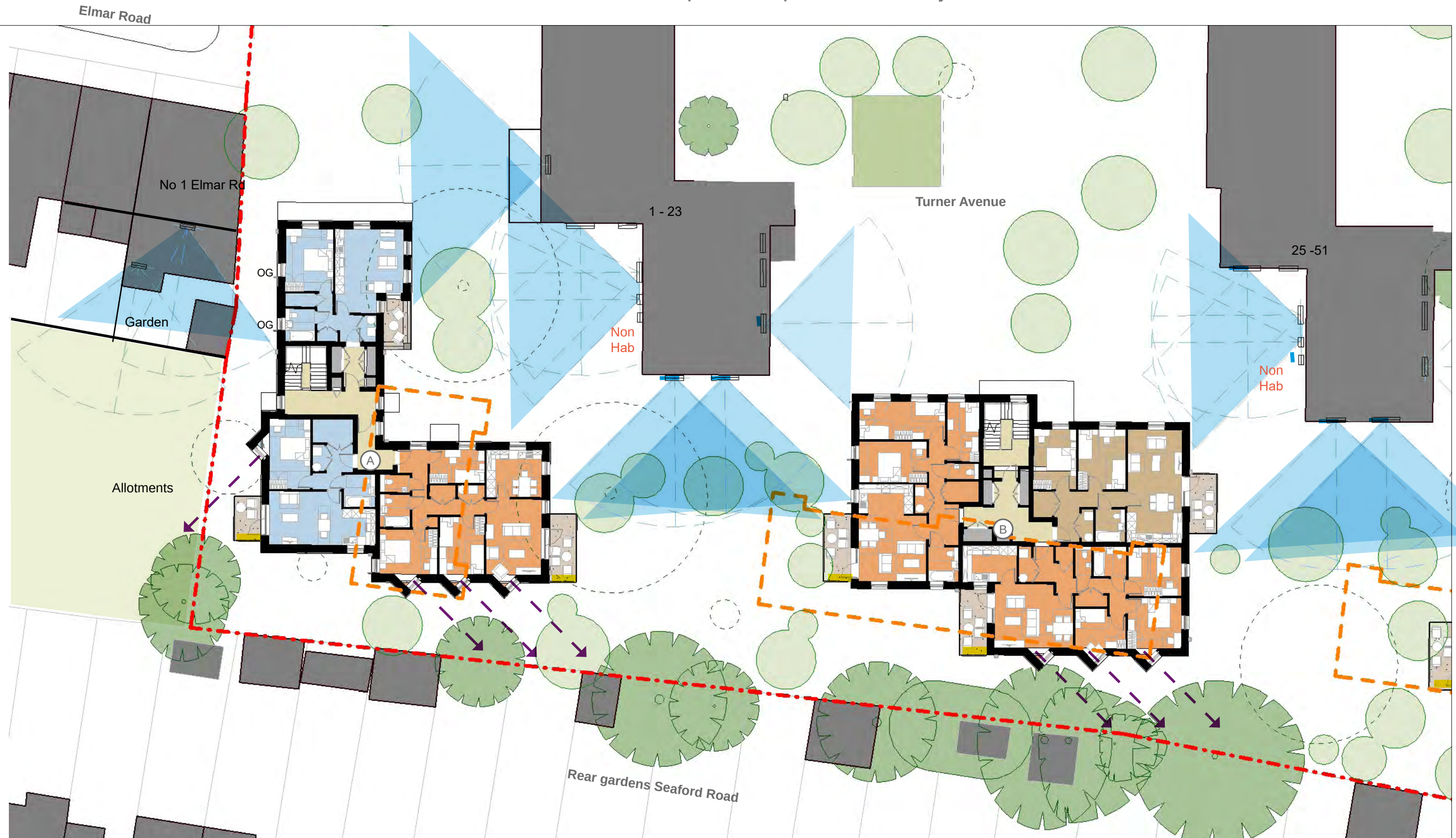
Proposed first floor plan - Blocks A + B. 1:500 approx @ A3
