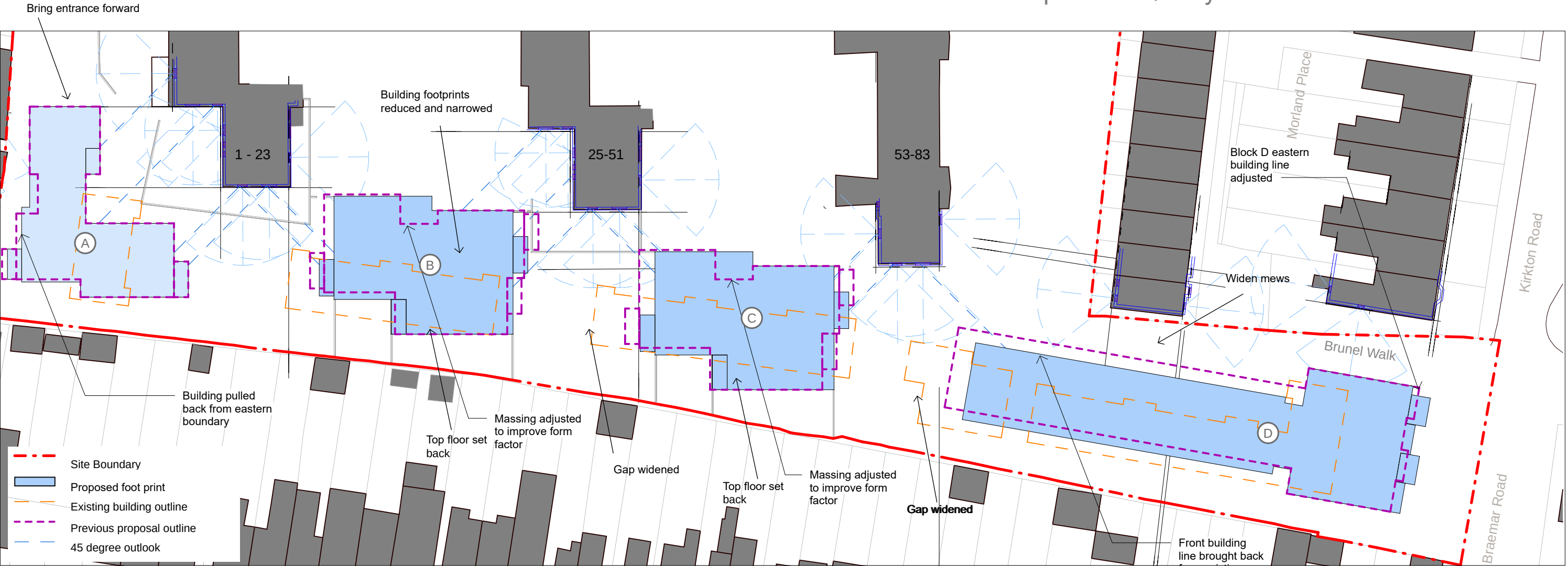
Revised Pre-app' 3 scheme compared to previous Pre-app' 2 scheme highlighting changes made - 1:500
