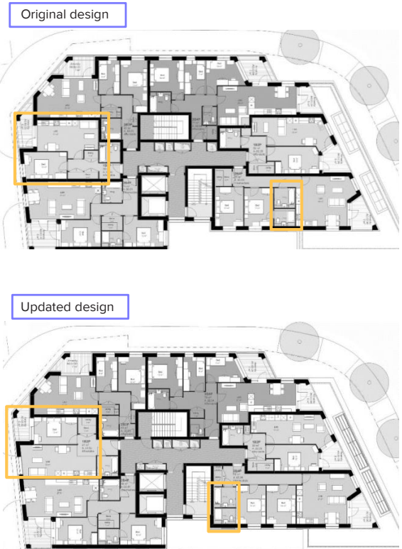
Figure 2: Demonstration of change in layouts to allow for better daylight penetration
