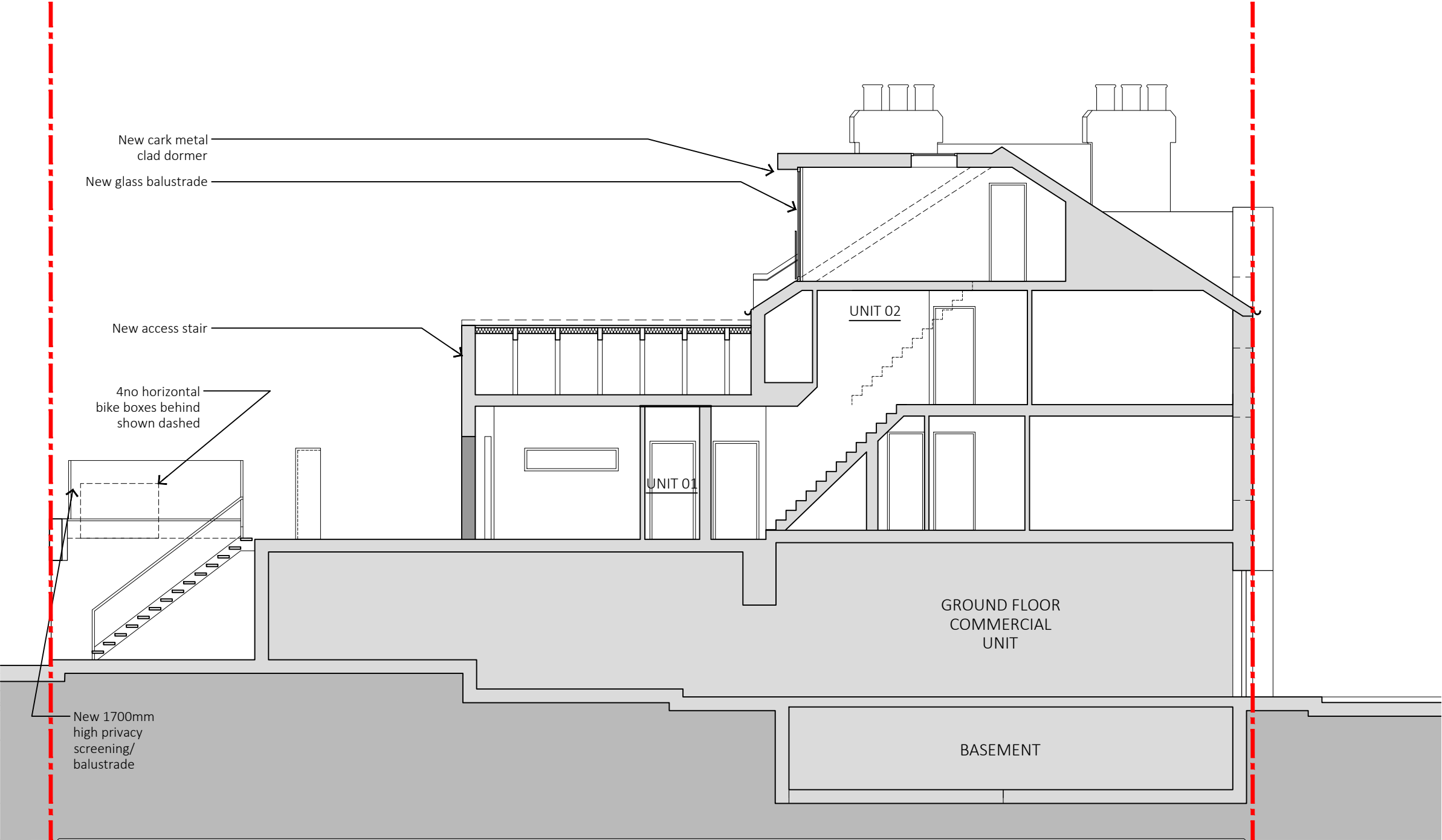
1 Proposed Section A:A 1:100 @ A3
