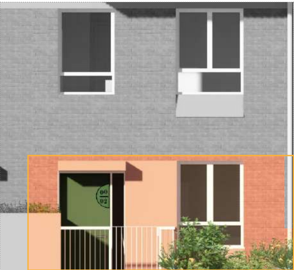
Duplex ground floor window with 675mm cill
