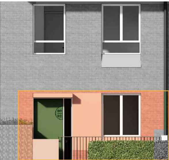
Duplex ground floor window with 1100mm cill
