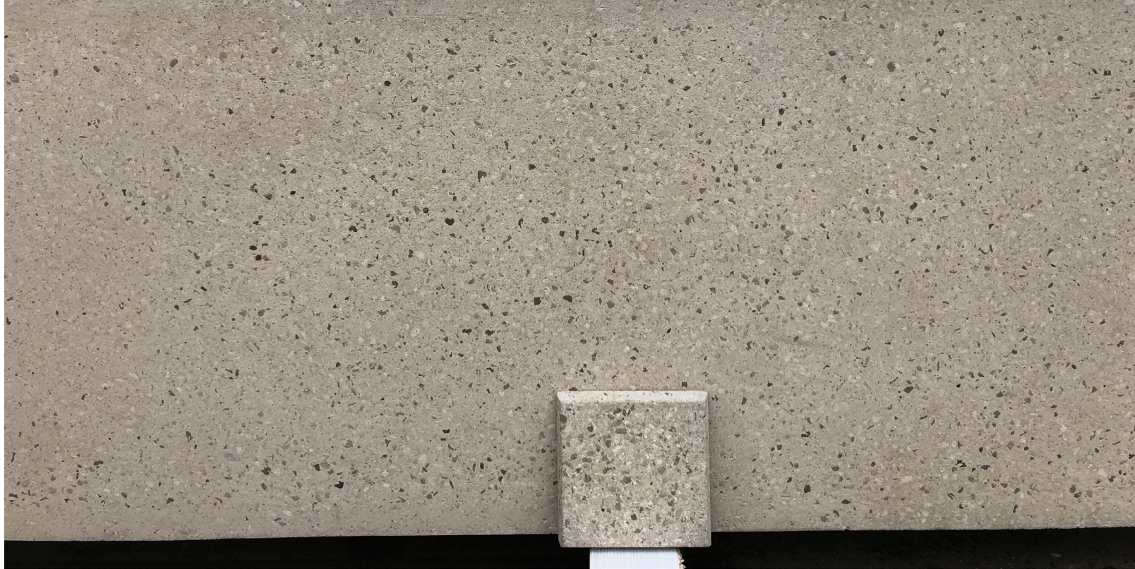
Pre-cast concrete lintel in the factory against a sample of Welsh Grey Very Heavy Etch
