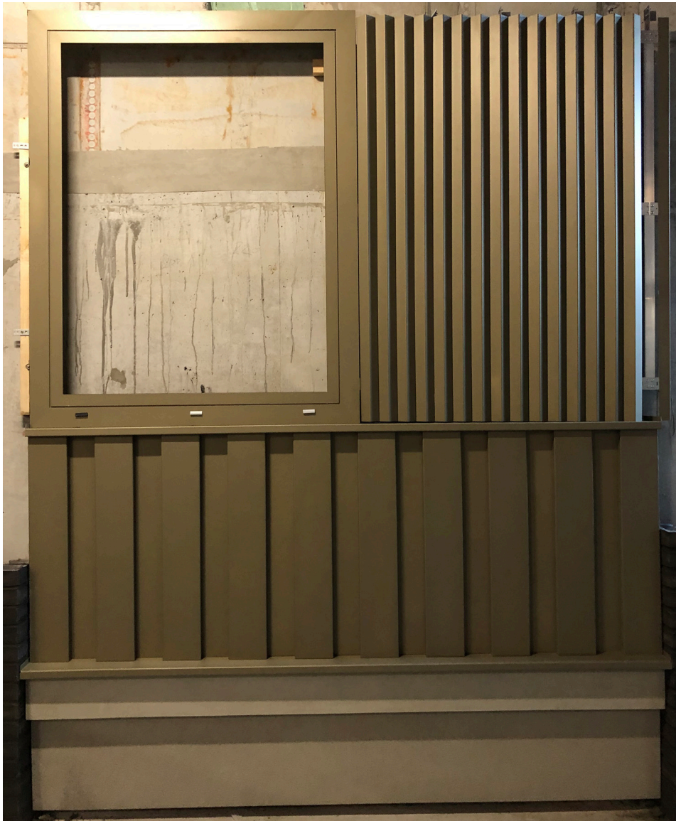
Rainscreen system & GRC mock-up with window frame
