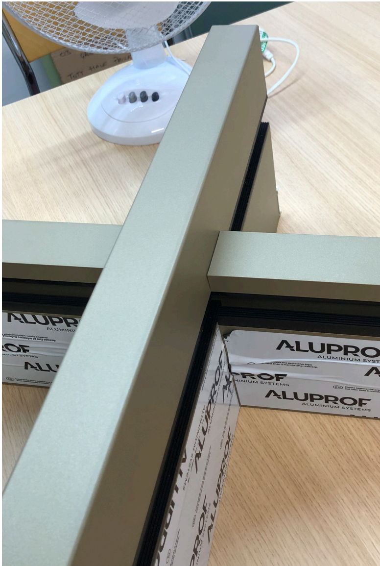
Sample of the curtain walling frame (under artificial light)
