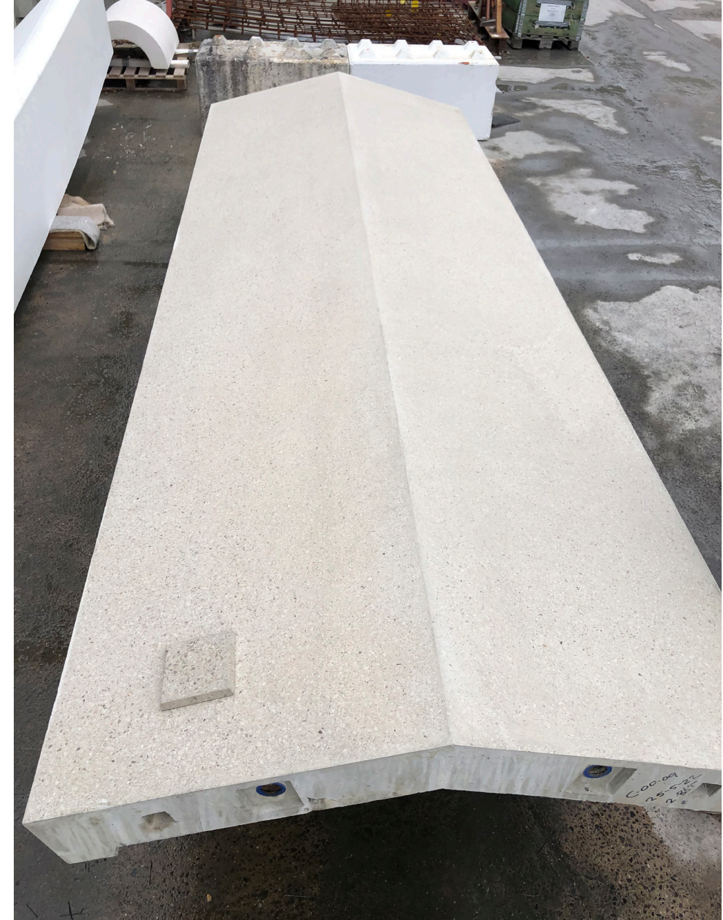
Pre-cast concrete angled pier in the factory with a sample of Welsh Grey Very Heavy Etch
