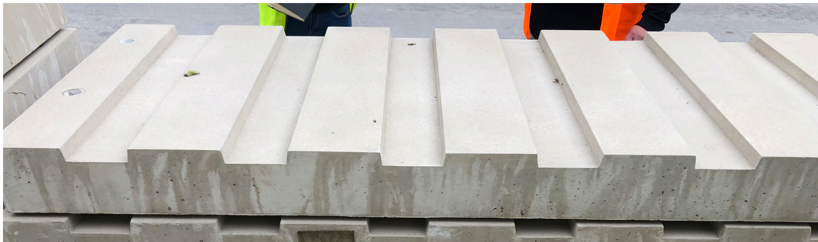
Pre-cast concrete profiled plinth in the factory (Welsh Grey Light Etch)
