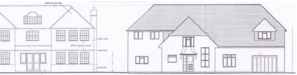
6. Appearance of the front elevation following the demolition of most of the two-storey east wing to create space for the construction of the new two-storey detached house next door at 27A Aylmer Road under planning permission HGY/2009/1002.
