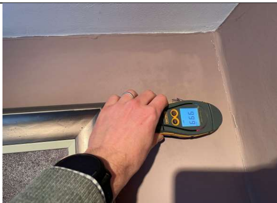
Images 12 & 13- Typical view of staining in Bedrooms 1 & 2 with positive moisture readings being taken on the return of the chimney breasts in both rooms
