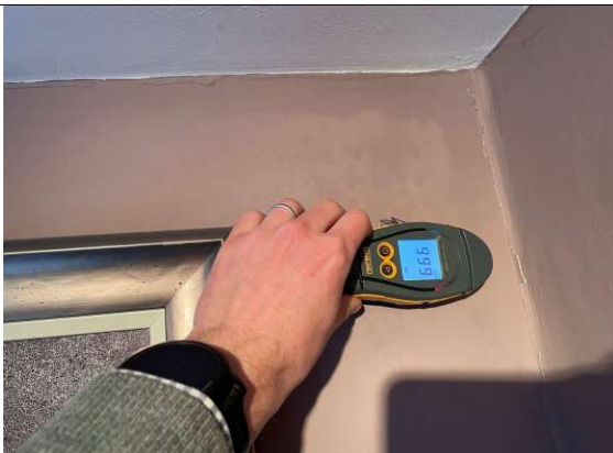
Images 13 & 14- Typical view of staining in Bedrooms 1 & 2 with positive moisture readings being taken on the return of the chimney breasts in both rooms
