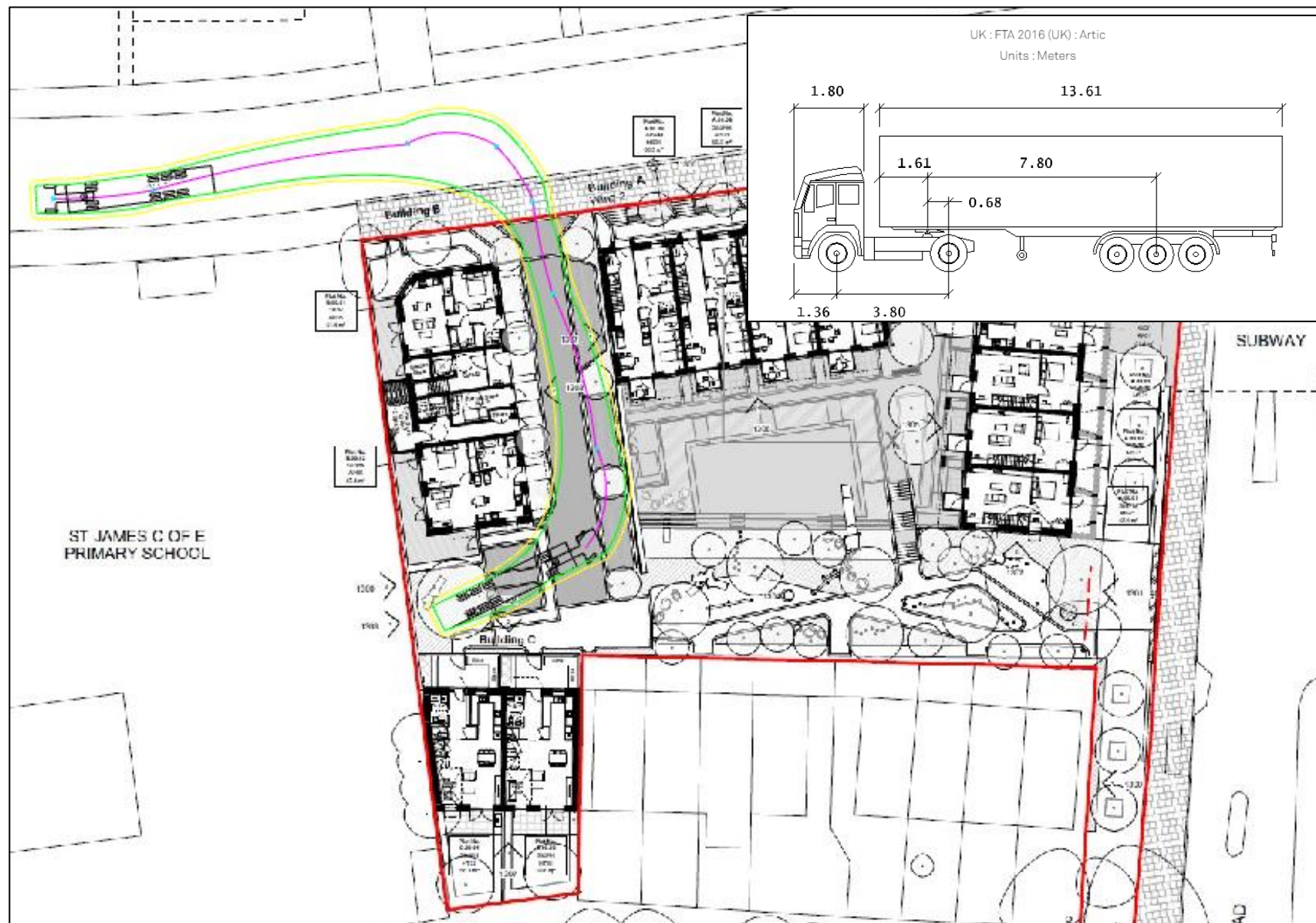
Figure 7.2(b): Construction Vehicle Egress
