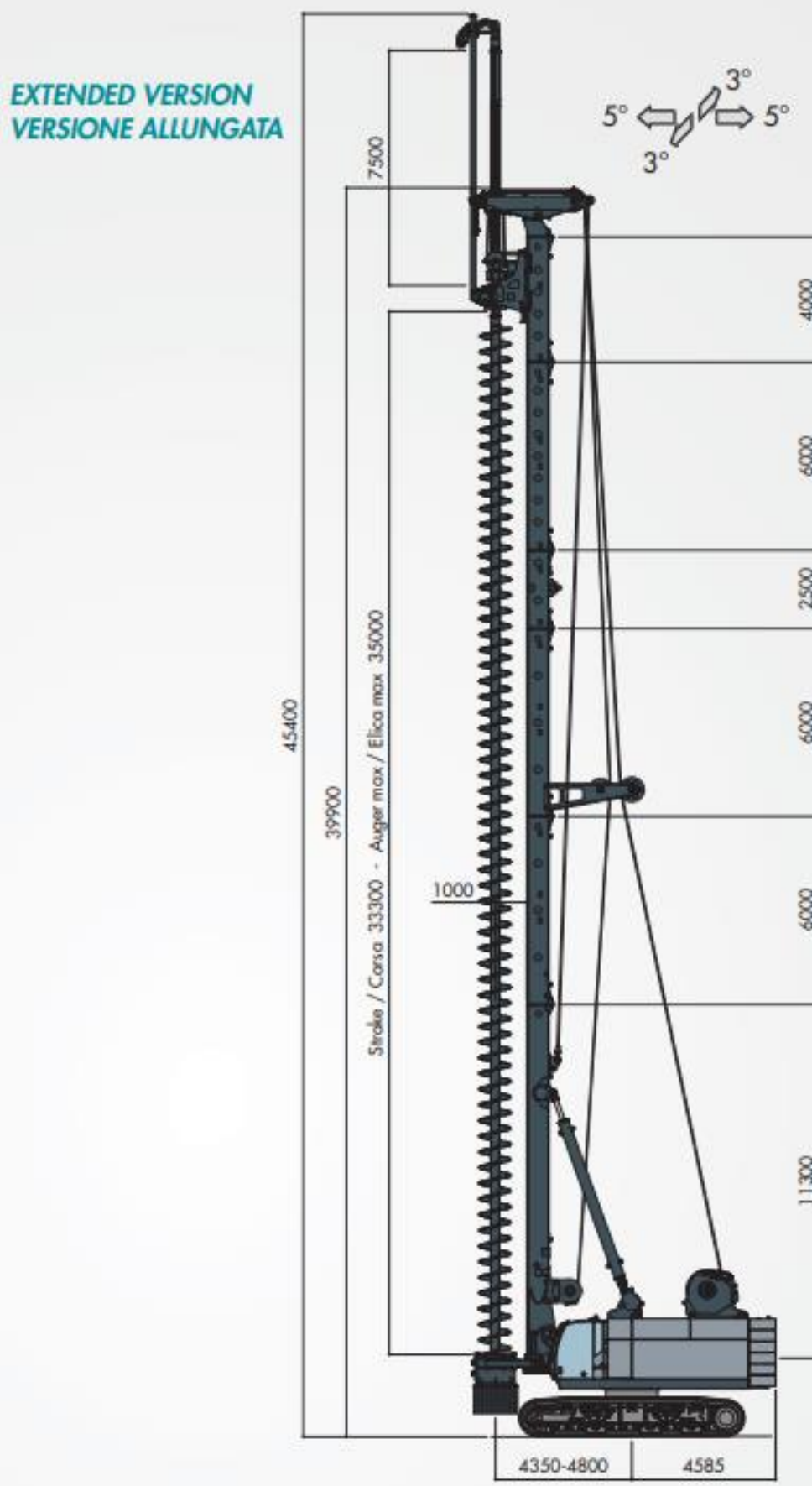
Figure 7 : Casagrande B470 XP2 in CFA mode
