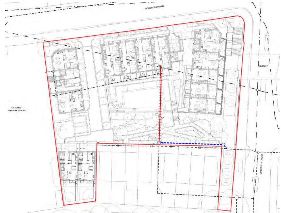
Figure 50. The existing upstream Thames Water manhole, located in Muswell Hill Road, is shown to have an existing connection into the foul water sewer in the highway. It is therefore considered that proposing a connection into the Thames Water foul water sewer will not be rejected.
