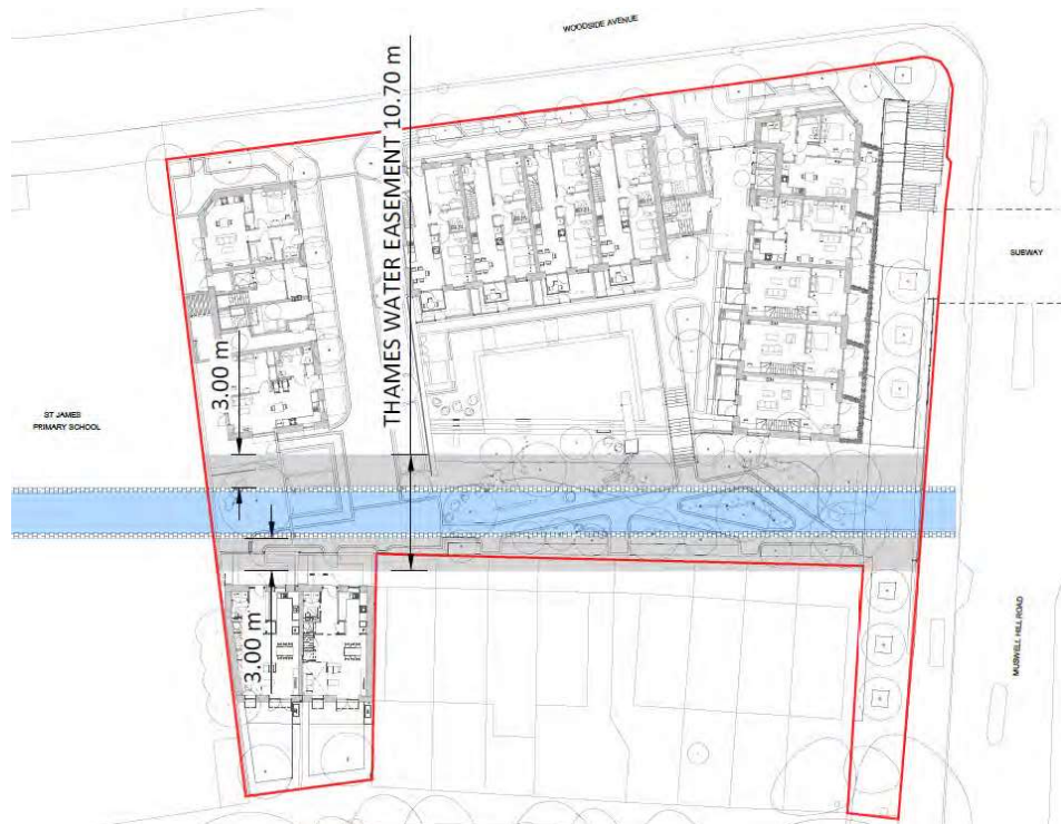
Figure 42 Thames Water trunk mains tunnel easement
