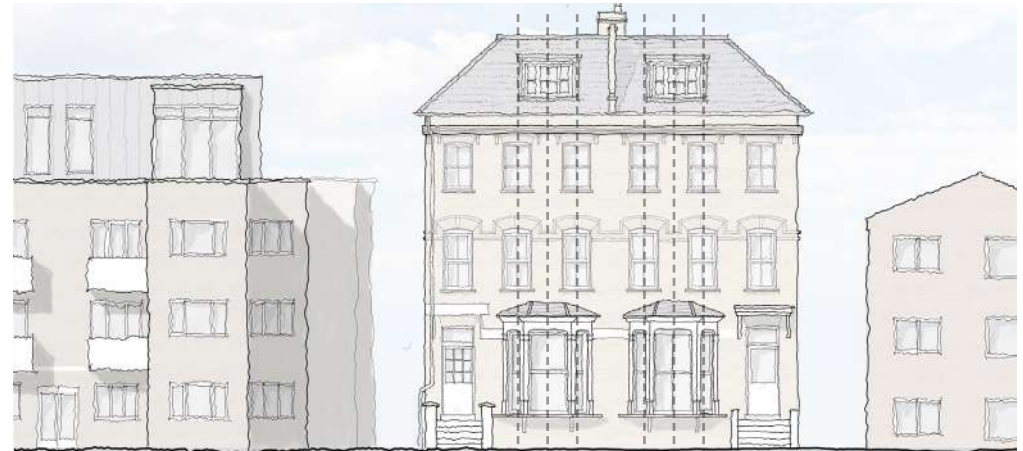
Sketch 1 - Proposed Front Elevation - alignments with the fenestration below
