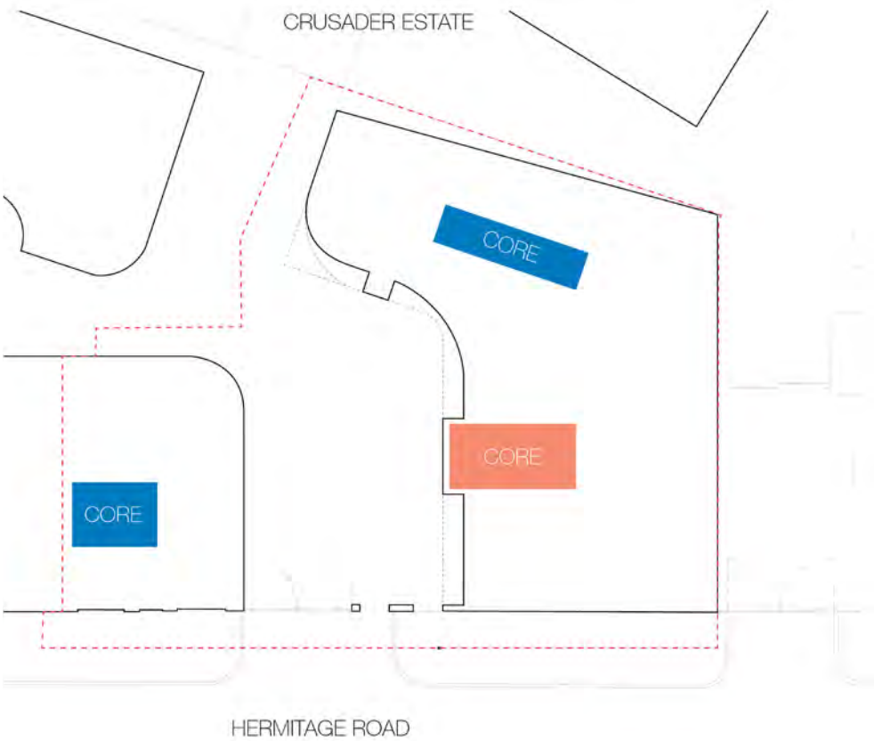
Residential and commercial stair and lift cores
