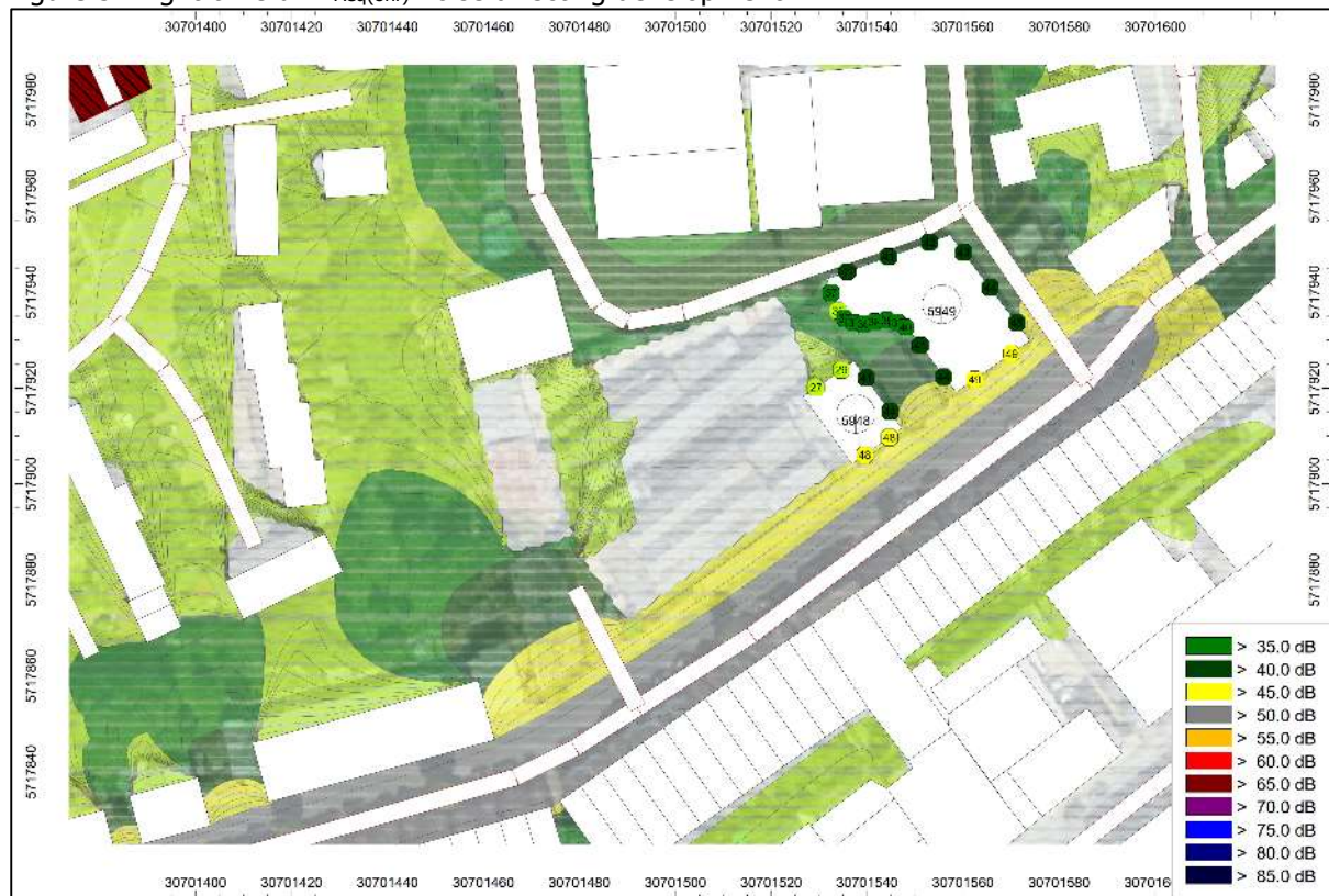
Figure 5: Night-time dB LAeq(8hr) noise affecting development
