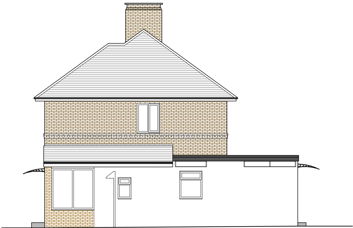
EAST ELEVATION (as existing)
