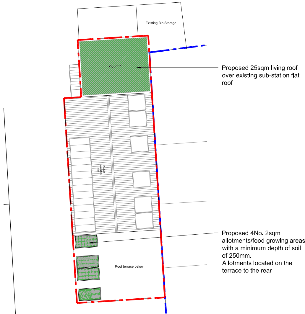
ROOF PLAN - Living roof location SCALE 1:200
