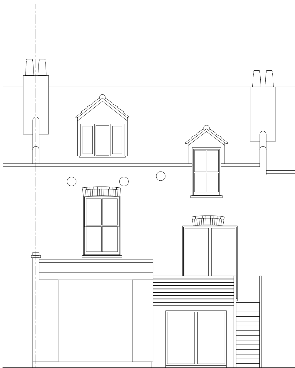
Proposed Section 1-1 (Rear Elevation)
