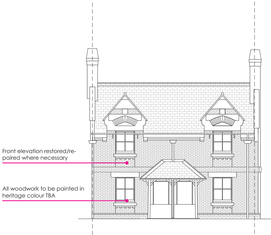
FRONT ELEVATION PROPOSED
