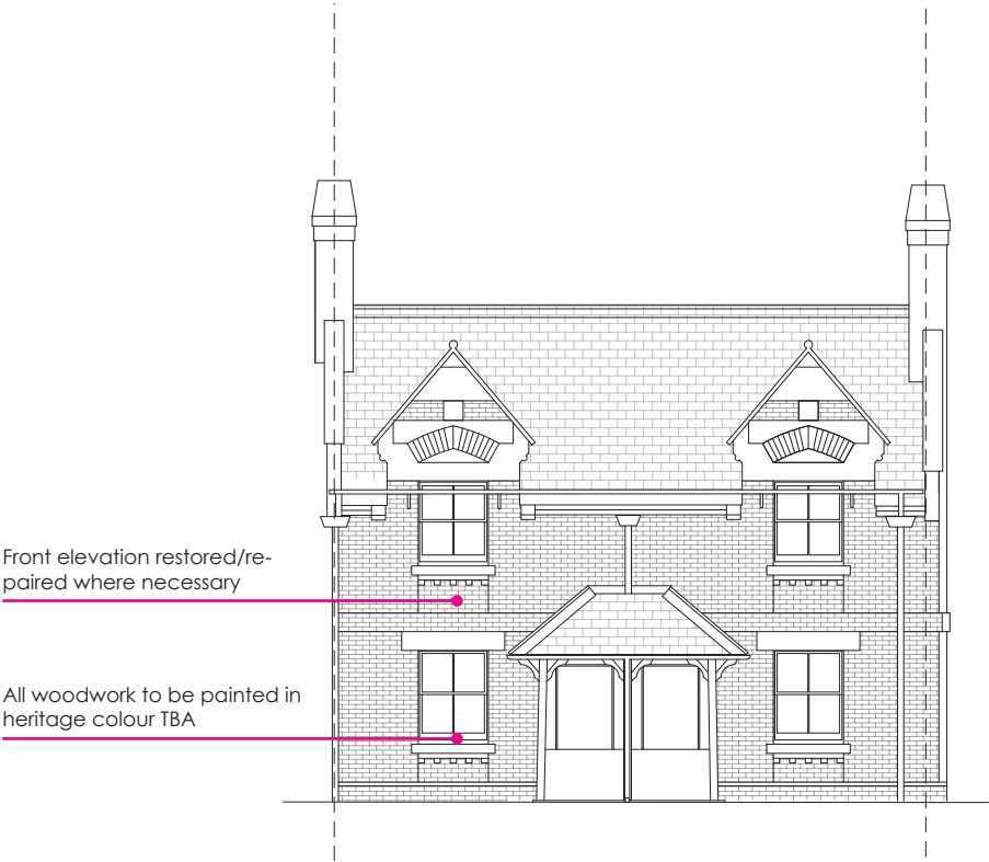
FRONT ELEVATION PROPOSED
