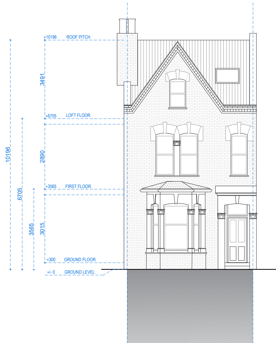
FRONT ELEVATION WEST ELEVATION
