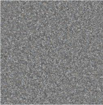
6. RESIN BONDED OVER PV PANEL ARRAY AREA
