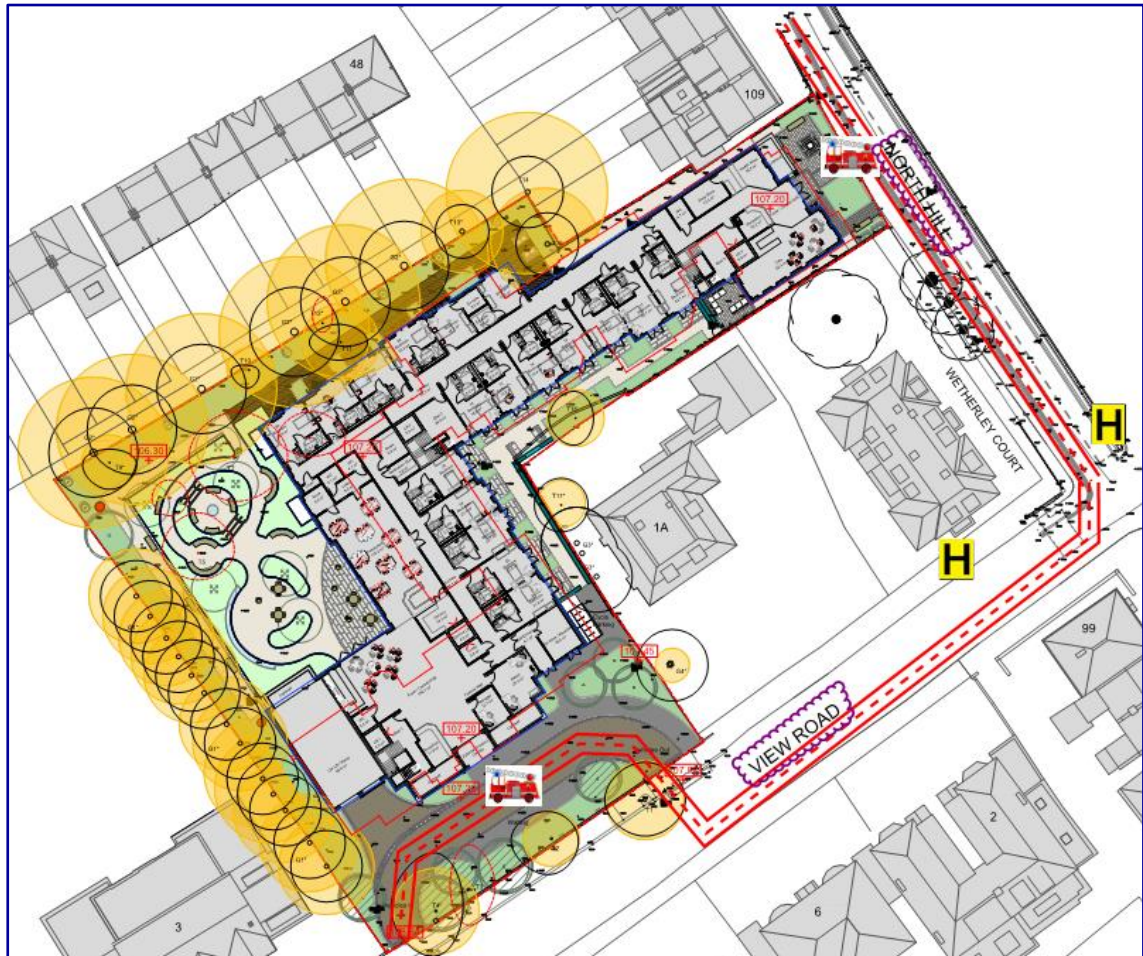
Figure 2 Fire Service Access, Hard Standings & Hydrants
