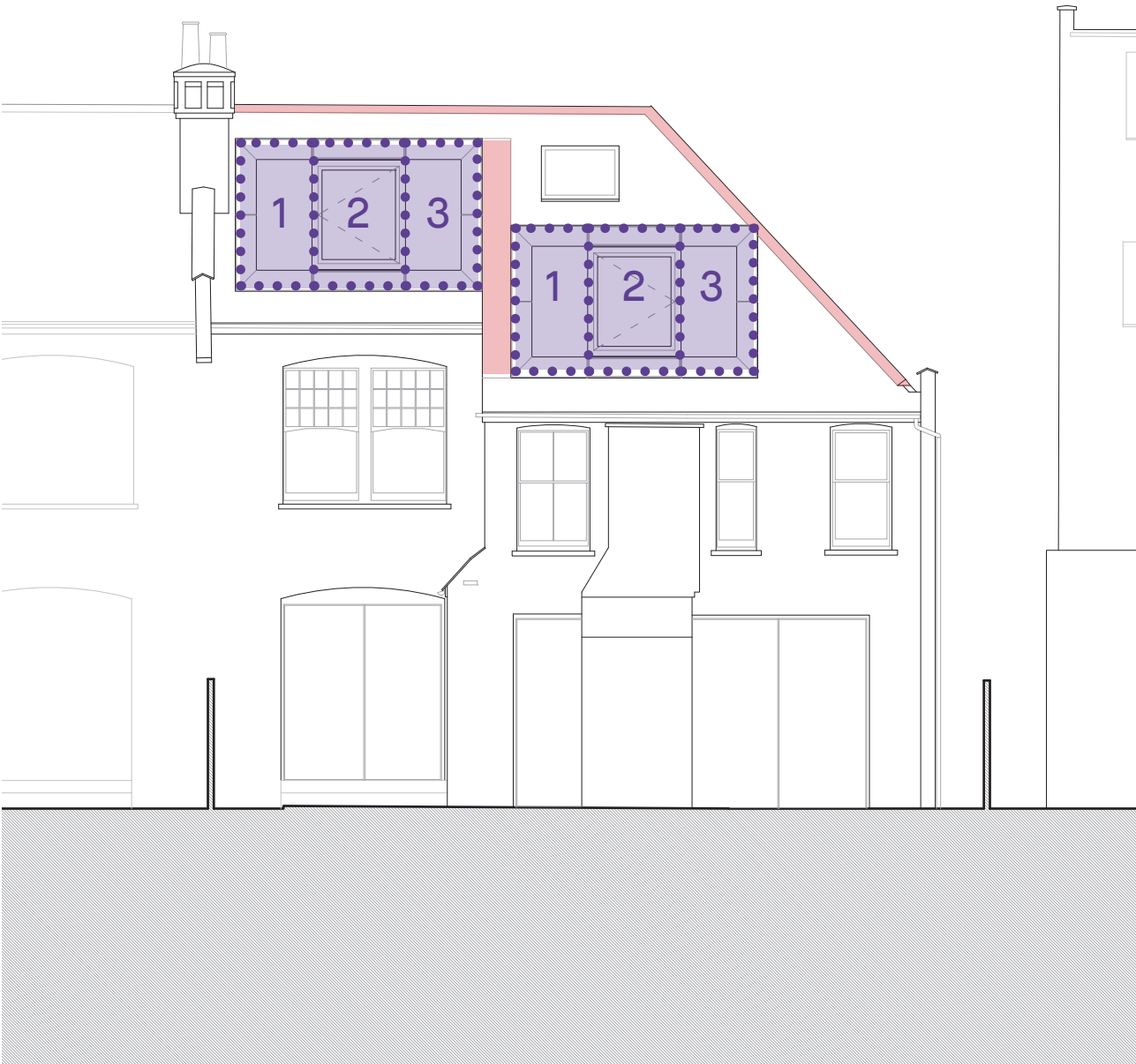
PROPOSED REAR ELEVATION - DECORATIVE RED FEATURES AND CENTRAL CONNECTING ELEMENT
