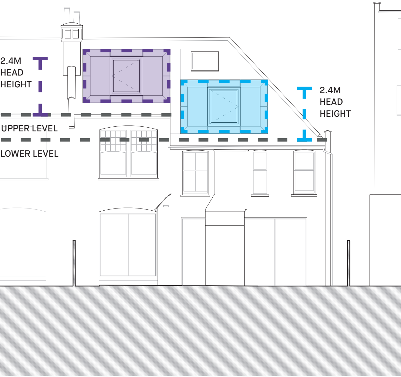
PROPOSED REAR ELEVATION - MAXIMISING HEAD HEIGHT
