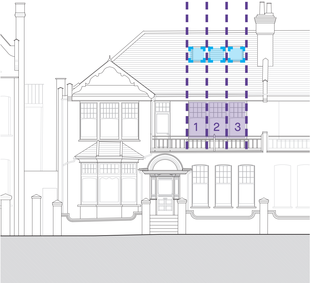
PROPOSED FRONT ELEVATION - ALIGNED ROOFLIGHTS
