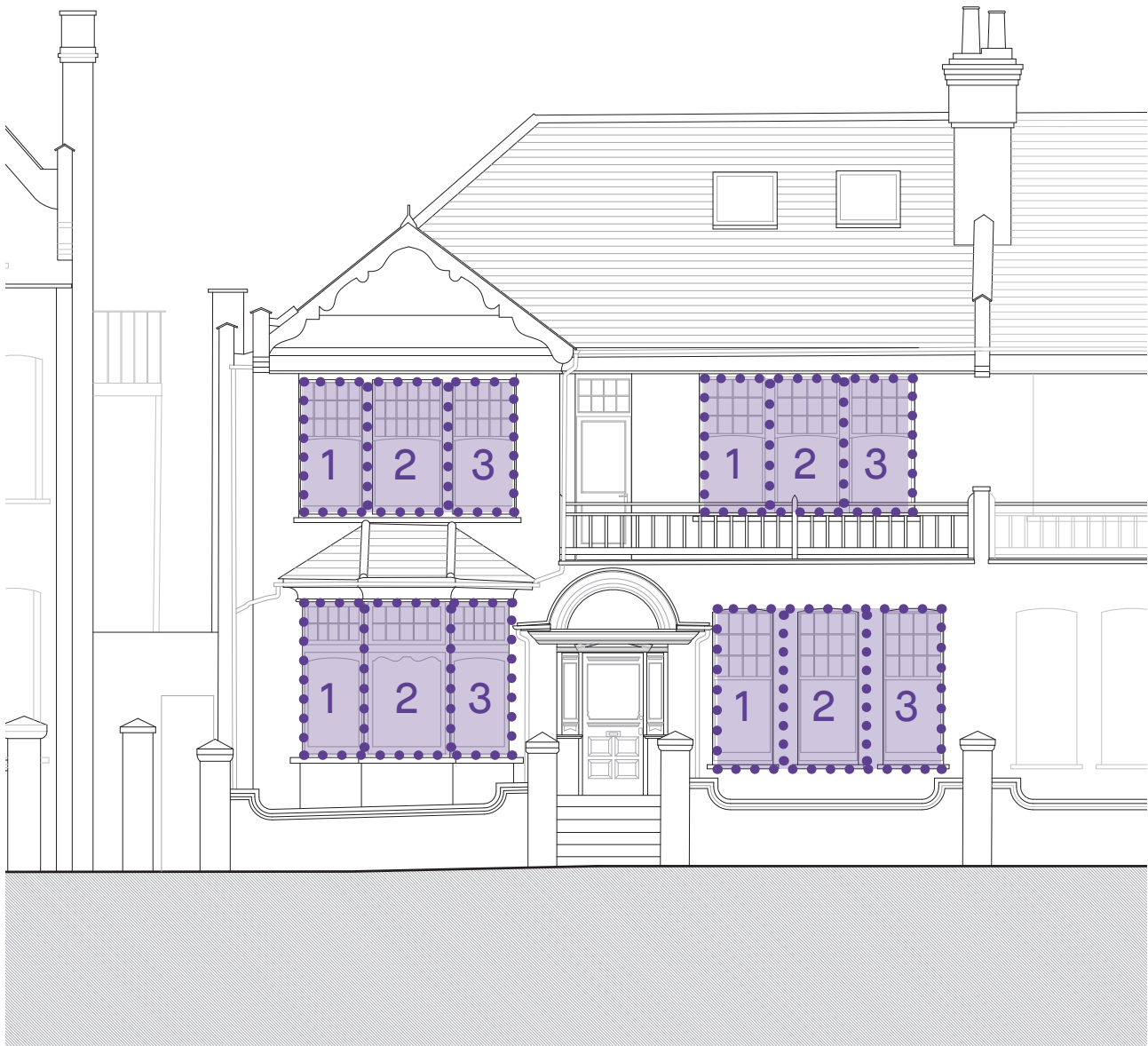
EXISTING NORTH ELEVATION - TRIPTYCH PROPORTIONS
