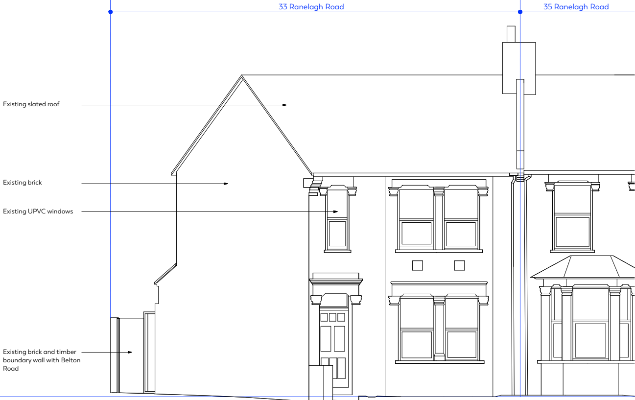
Existing Front Elevation
