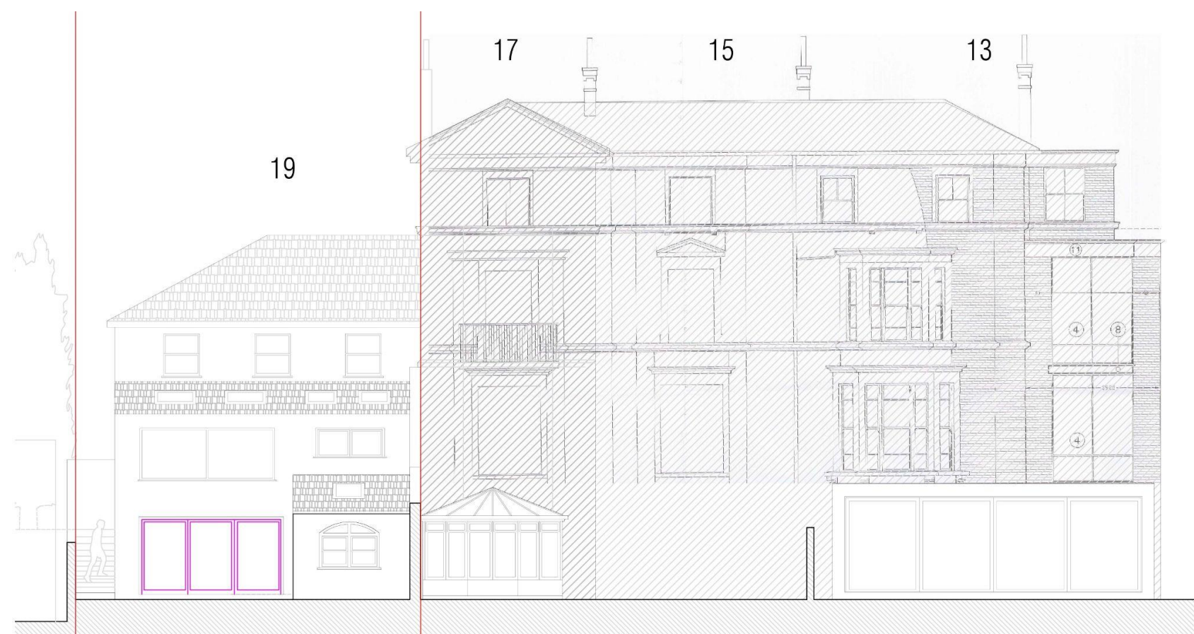
Proposed Rear Elevation (extract) showing proposed doors at no. 19 (outlined pink), relative to the block and glazed doors at no. 13
