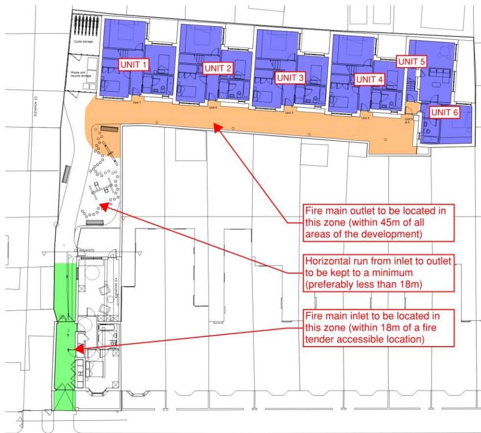
Figure 3 Proposed fire main location
