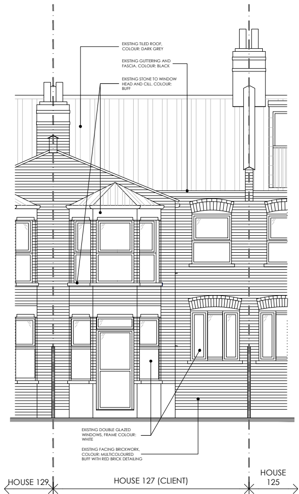
EXISTING REAR ELEVATION | 1:100
