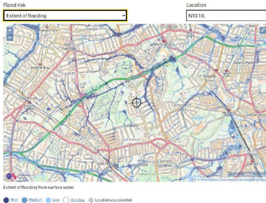
Figure 20 - Extent of flooding from surface water
