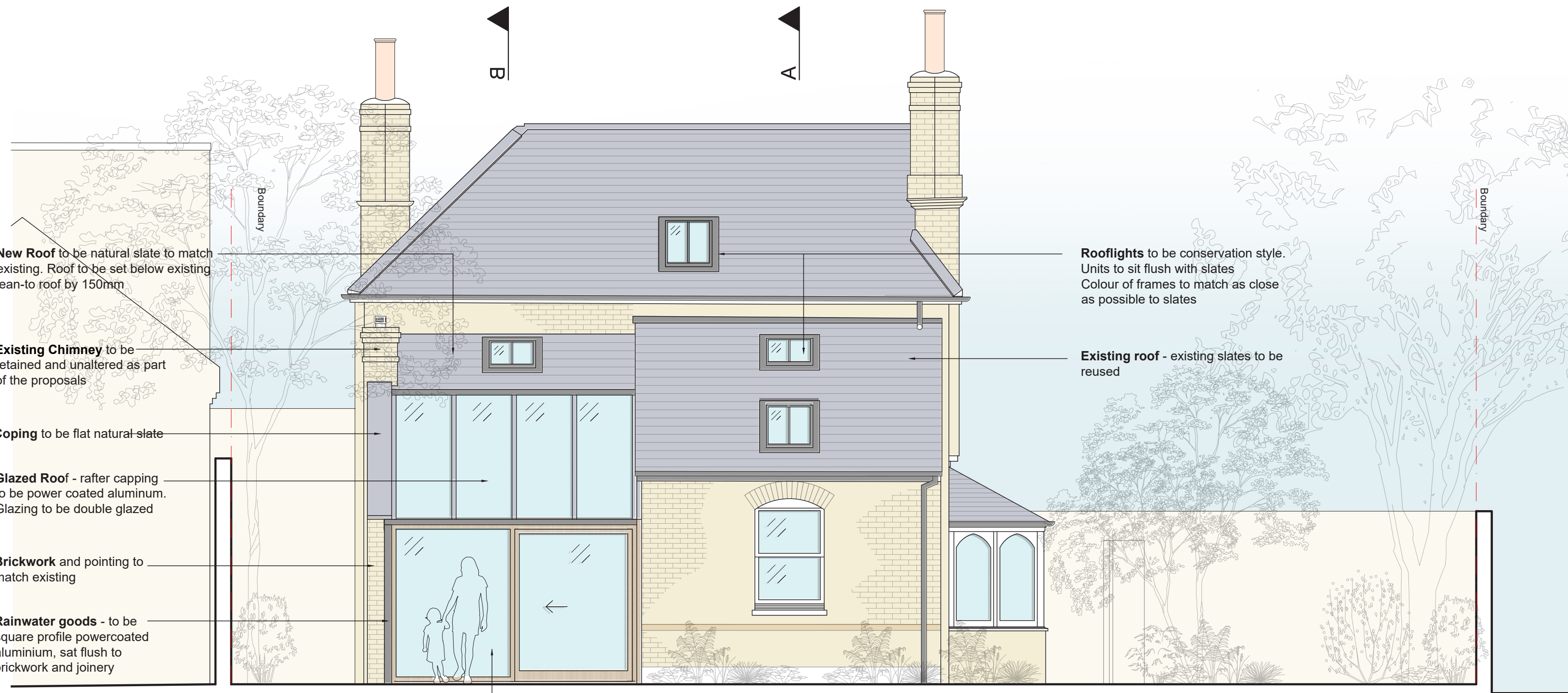
SOUTH-WEST ELEVATION AS PROPOSED
