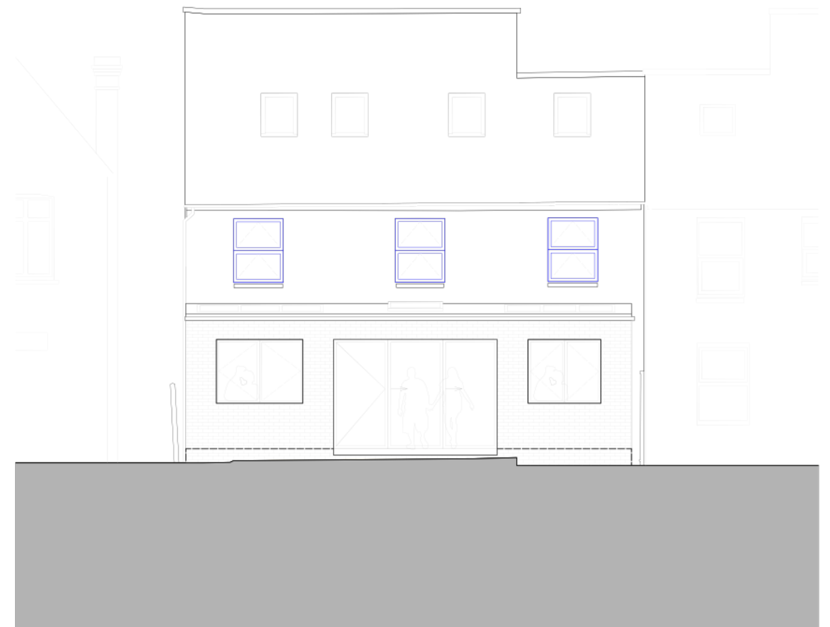
Rear Elevation highlighting the uPVC windows to be replaced on 1F
