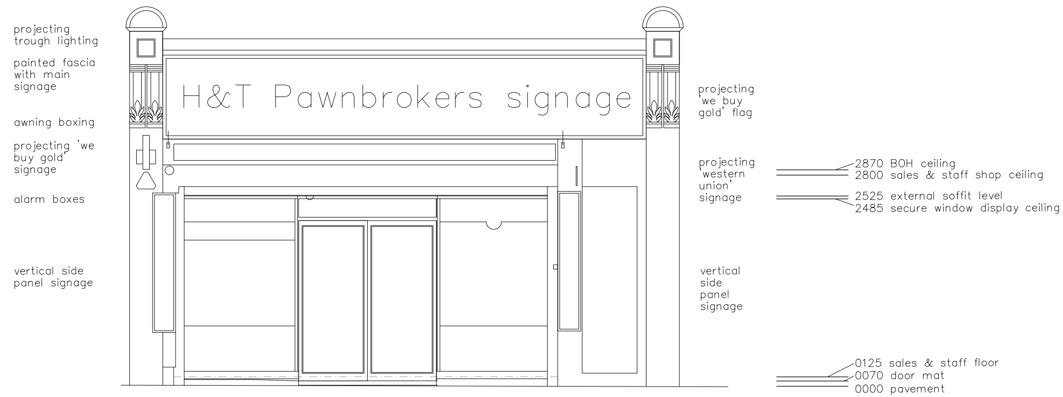
EXISTING SHOP FRONT ELEVATION
