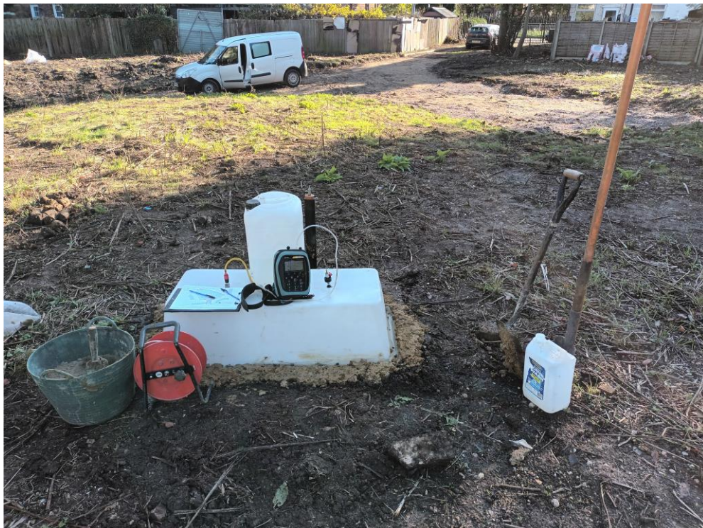
Showing flux box tested area FLB03 adjacent on top of a mound of soil near the previously drilled CT03.
