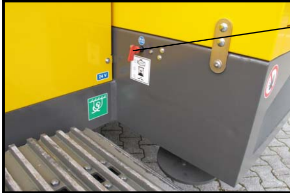
Battery main switch
