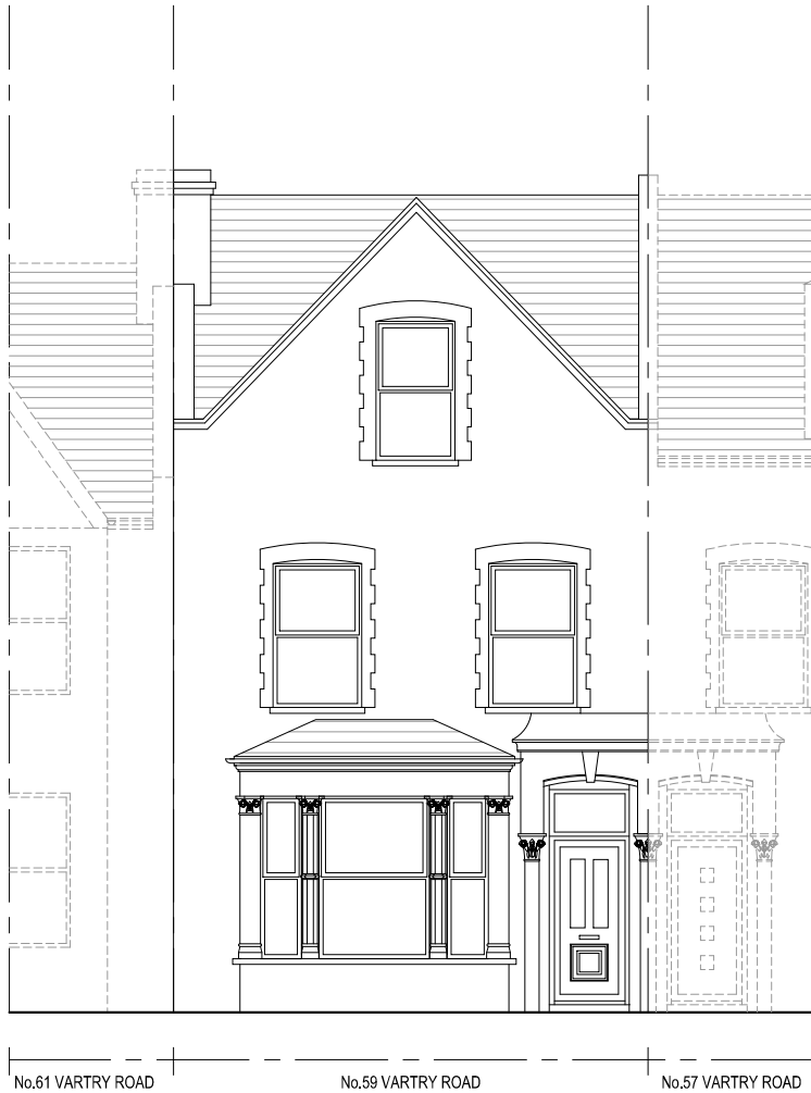
EXISTING FRONT ELEVATION
