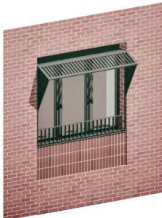
Figure 6-2 Shading design - Horizontal and vertical shading to both vertical reveals
