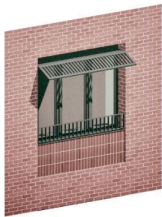
Figure 6-1 Shading design - Horizontal and southern vertical reveal
