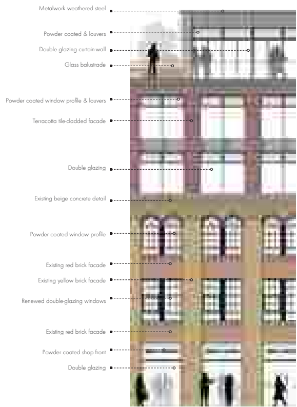
Figure 8: Berol House facade treatment
