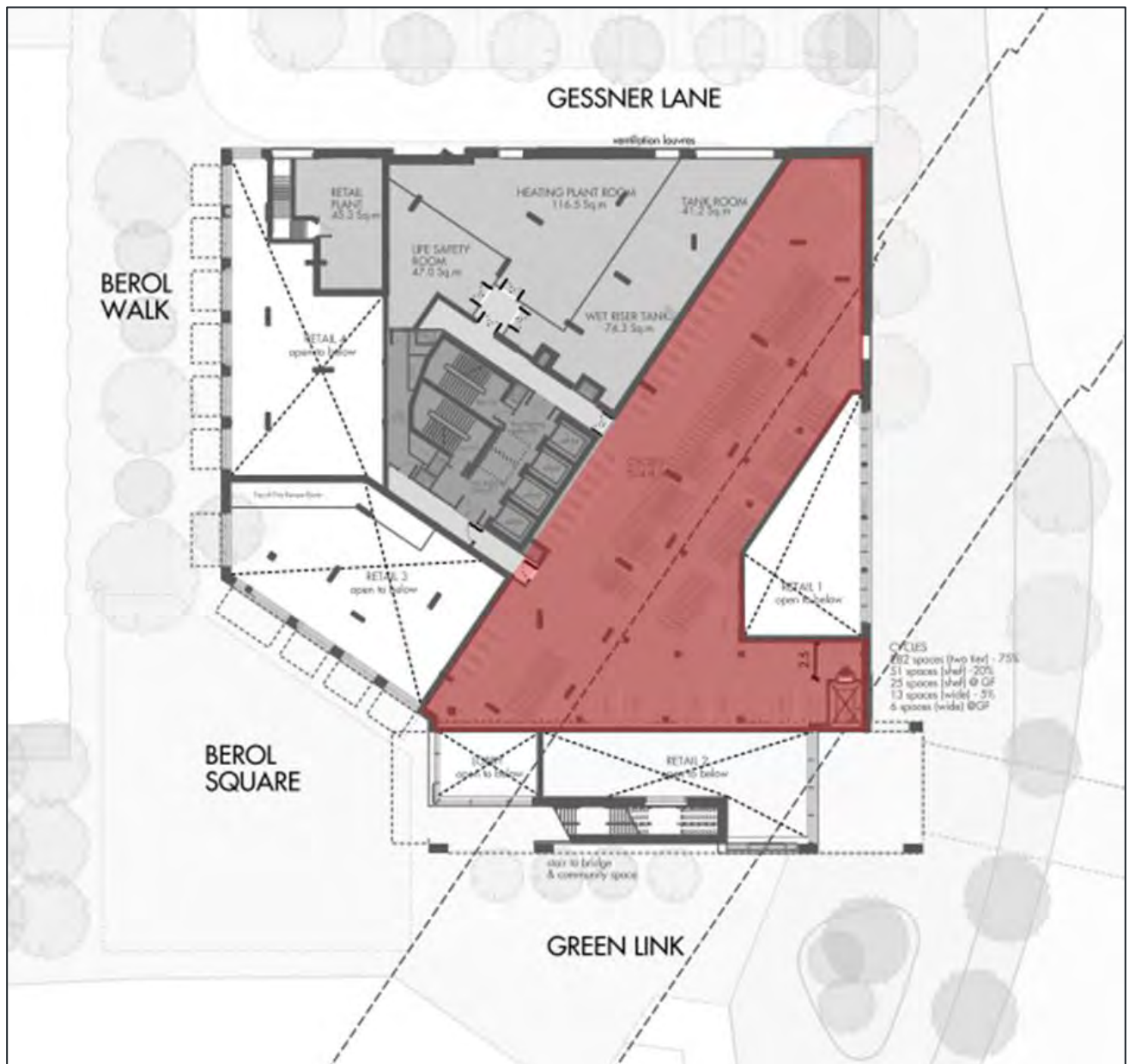
Figure 6-7 2 Berol Yard Mezzanine Floor Cycle Facilities
