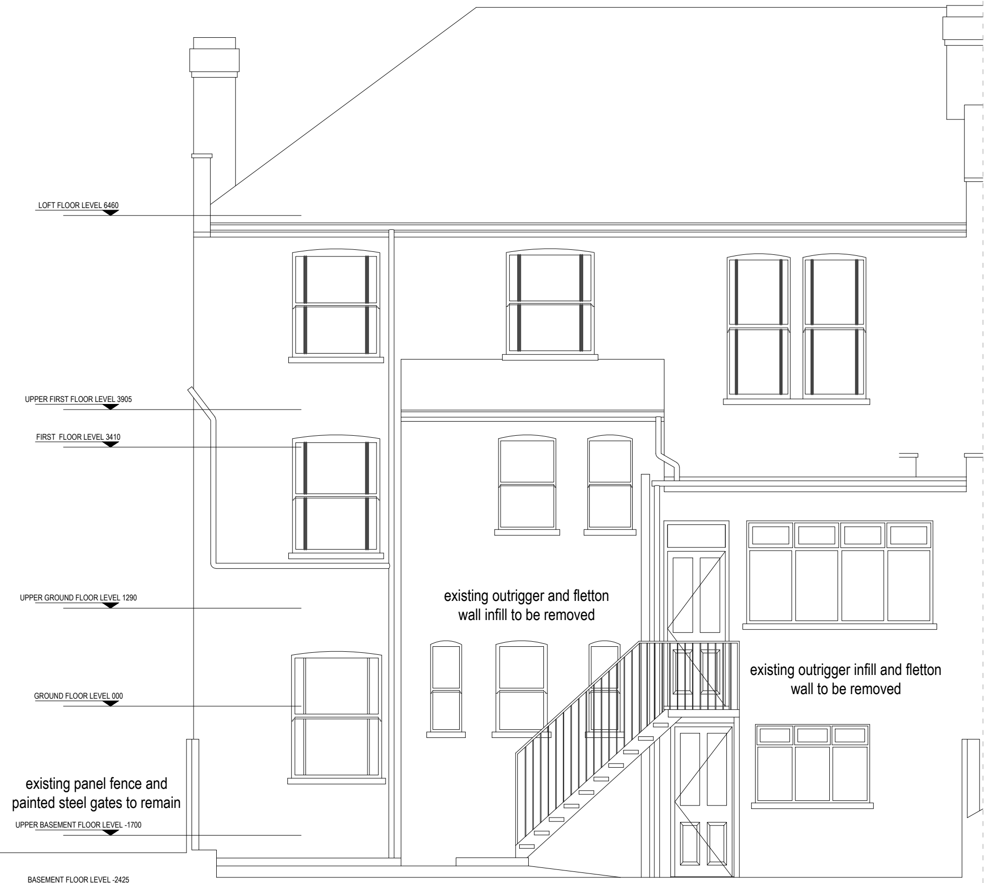
EXISTING REAR ELEVATION
