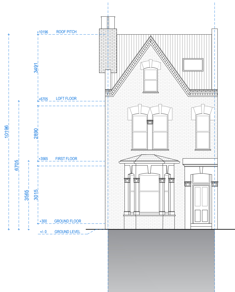
FRONT ELEVATION WEST ELEVATION
