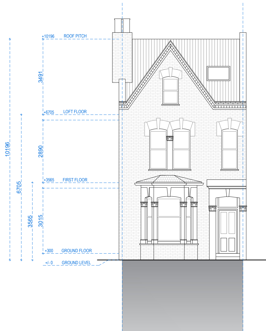
FRONT ELEVATION WEST ELEVATION
