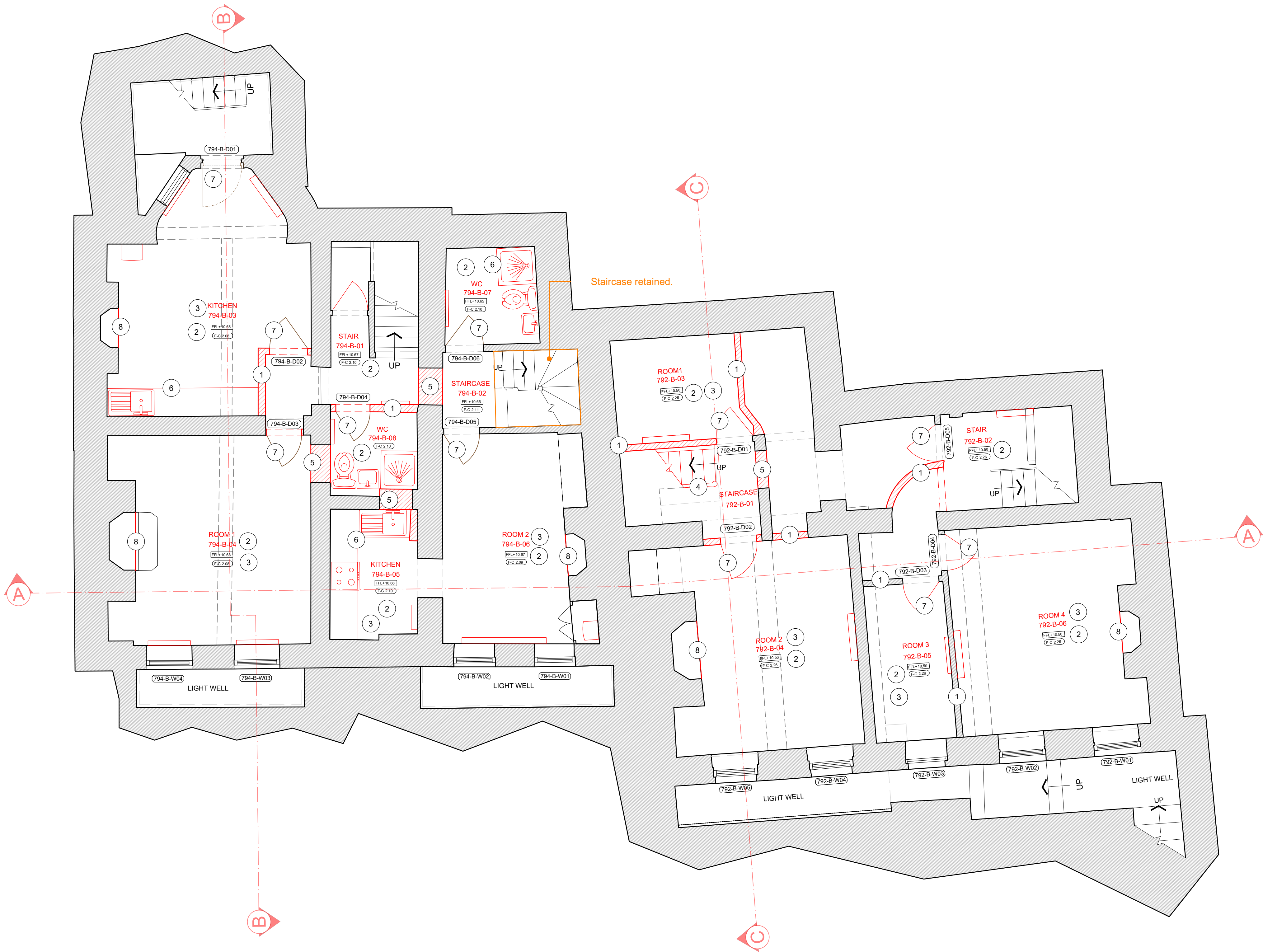
01 EXISTING + STRIP OUT BASEMENT PLAN 92210 Scale 1:50
