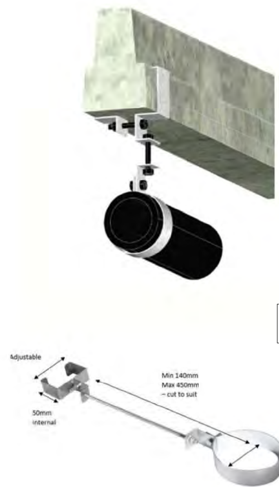
BLOCK & BEAM DRAINAGE HANGER
