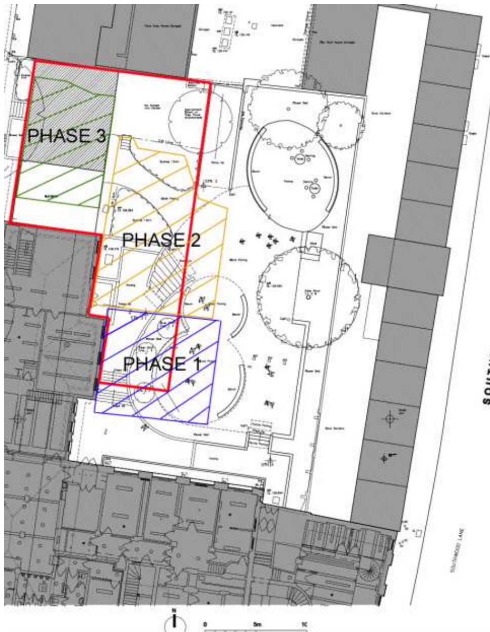
Fig.12: Plan of the redevelopment site, with the extent of excavation shown in phases
