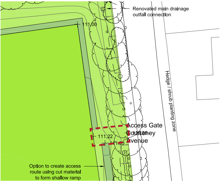
Fig. 36: Grass reinforcement proposed for existing entrance via Courtenay Avenue
