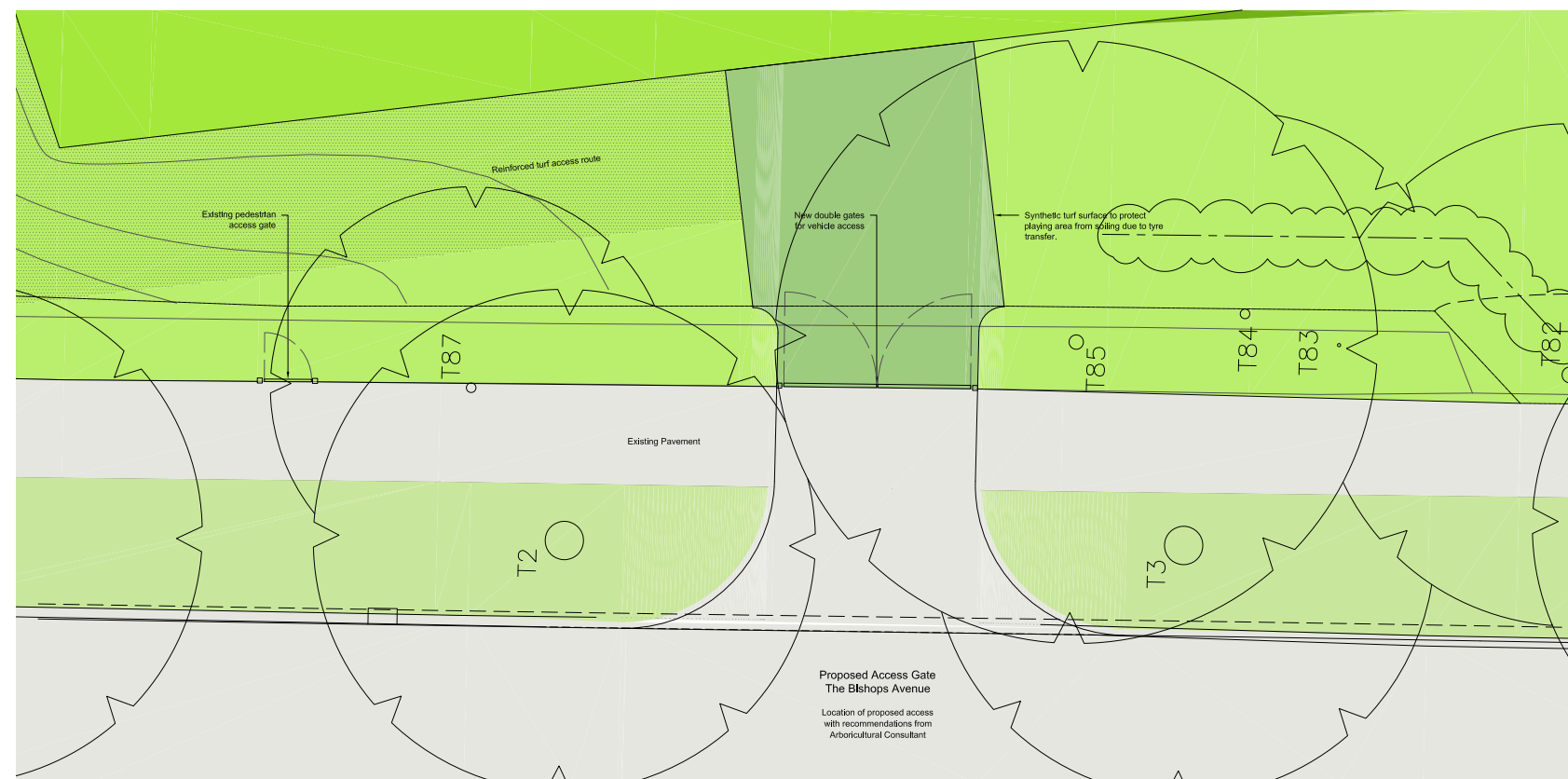
Fig. 33: Plan view of the proposed access off The Bishops Avenue, comprising a double gate for vehicle access. Gate to be fitted with self-closing device and to have mechanical keypad-type combination locks.
