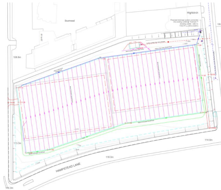
Figure 14 – Proposed Pitches and Embankment Drainage
