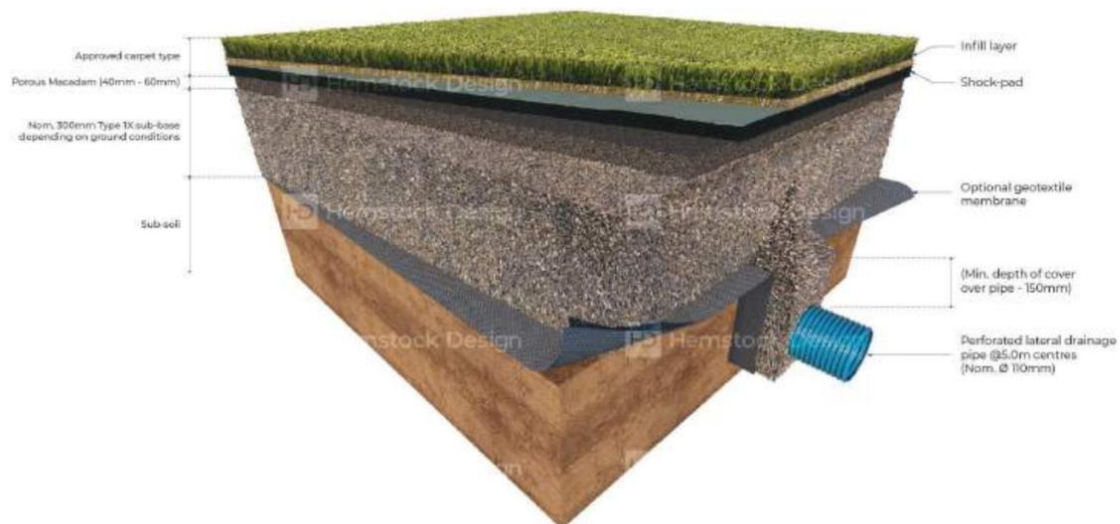
Figure 13 – Typical Synthetic Pitch Cross Section
