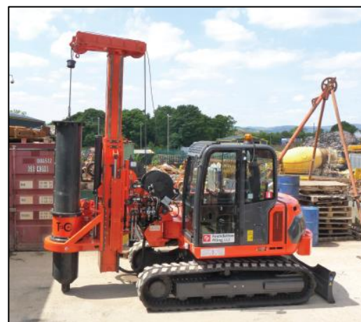
CF3 RIG, 2.2M WIDE, 11 TONNES
