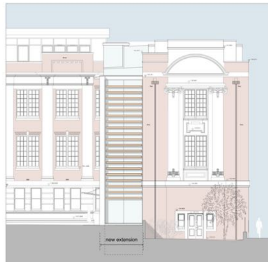
South elevation proposed with new extension
