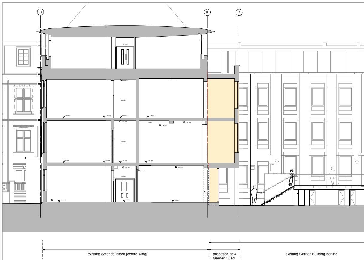
Section through Centre Block, with proposed extension shaded yellow
