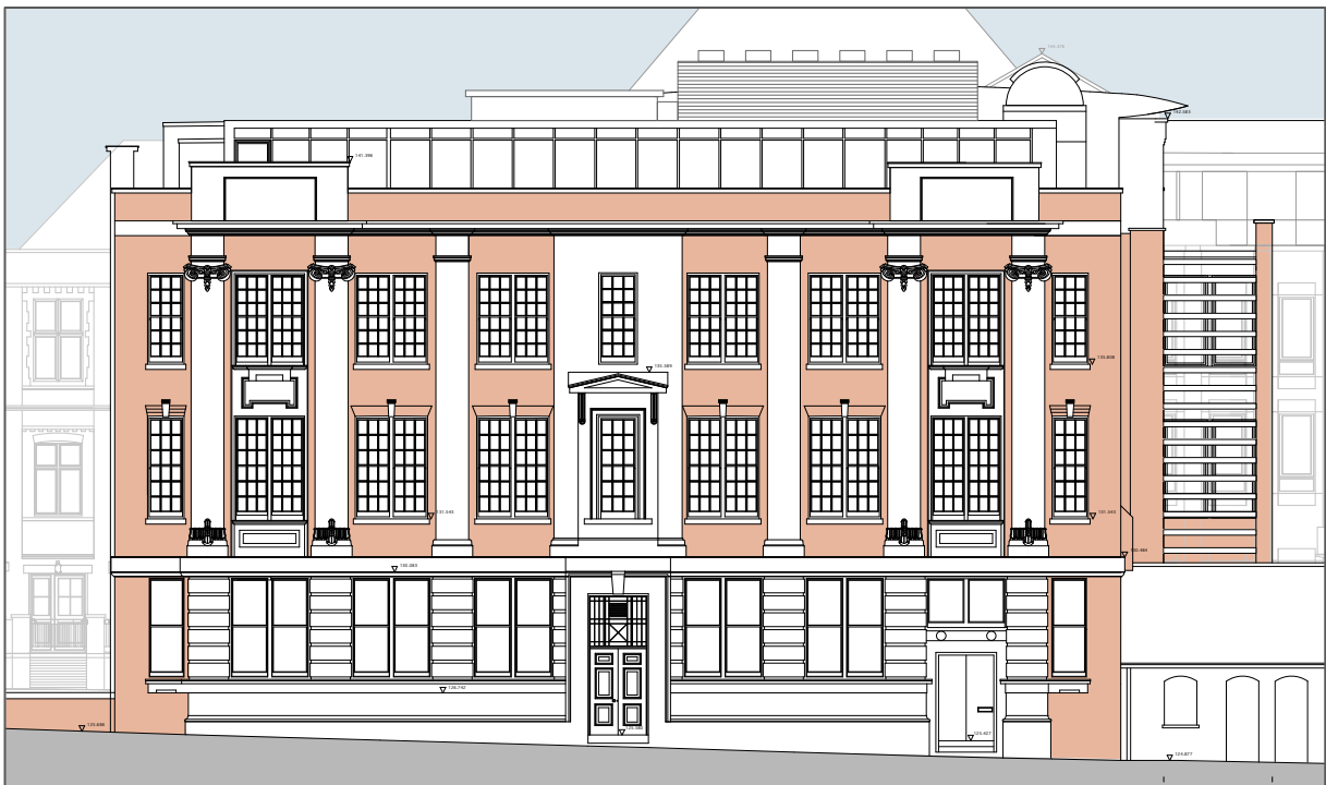
East elevation with rooftop plant area & observatory behind east block, north extension on right side
